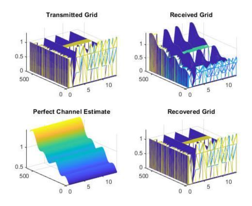
Comparing the transmitted grid to the recovered grid shows equalization of the received grid with the perfect channel estimate recovers the transmission.
