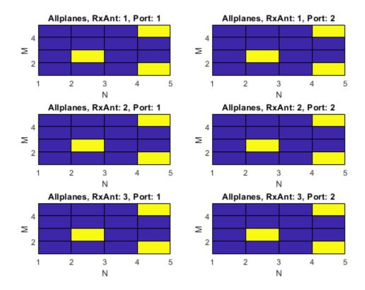
Create a 4D channel estimate grid to extract resource elements. Extract resource elements from the channel estimate grid using 'direct' extraction mode. Show the locations of these extracted resource elements. Addressed resource element locations contain 1.
